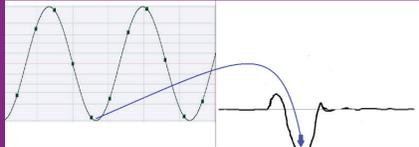
And indeed, this is what the demodulated composite clipped signal looks like in the above example. As you can see, it is very close to the original signal, and the stereo difference has not been reduced as was the case for the left/right clipped signal.
