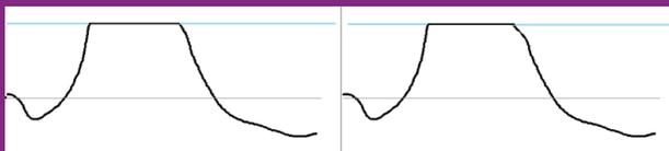
So, what do we do when we create a composite signal? Instead of working with the left and right channel, we are going to work with the L+R (just the mono sound) and L-R (the stereo sound, the difference between the two channels) signals. You can see what those signals look like on the right.
