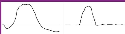
So, let us first check what happens in stereo modulation. Basically, the L-R signal is multiplied by a 38 kHz sine wave. Which means that there is a good chance that the resulting waveform is less loud (the average sample value is 3 dB's lower), and if it is short enough, there is a 50% chance that the resulting waveform points in the opposite direction.
