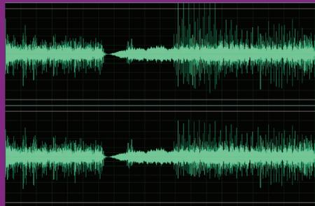
Here is the same audio, processed without Intellilimiter on top, and with Intellilimiter at the bottom. What is clearly visible is that not just the highest peaks got reduced (as a direct effect of the limiting), but lower peaks are also reduced. The end result is a more dynamic, less restrained sound. Also, short loud sounds may not have much effect on the measured level, but they still sound loud to our ears, so reducing them and everything around them sounds more natural.
