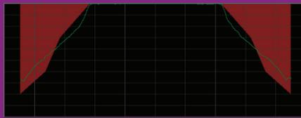
Without RF bandwidth protection. Each horizontal line is 10 dB, so the overshoots are close to 15 dB.
